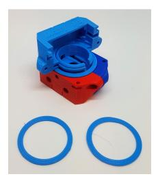
The thrust washer is placed in the middle of the knee assembly, as shown in the above photo
